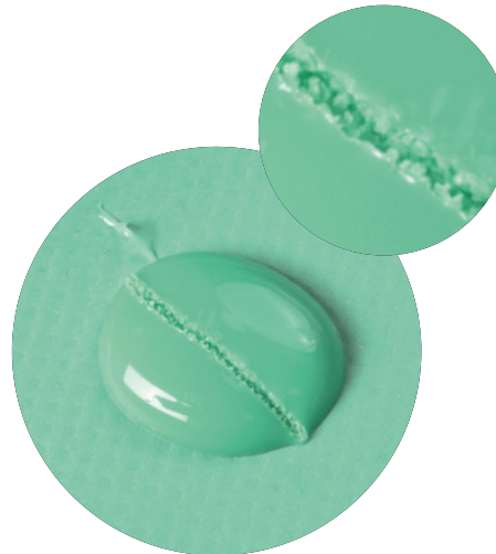
Fig. 38: Absence of an unpolymerized layer (smear layer) shows compatibility of the used materials.
